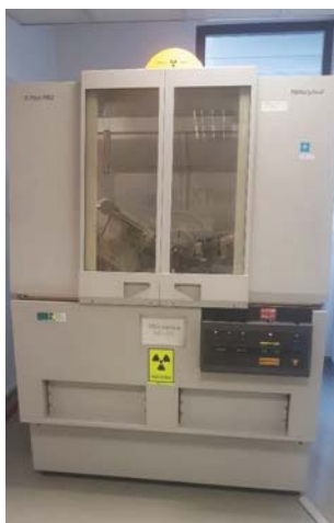
PANalytical X'Pert PRO CuK \alpha 1 – high resolution diffractometer (2005; D09/FKKT)
