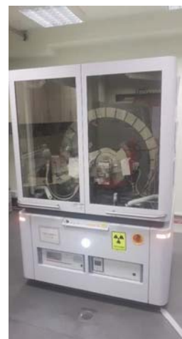
PANalytical Empyrean Cu, Mo, Ag X-ray source, modular setup, PDF analysis (2020; D09/D10/D13/FKKT, director's fund )
