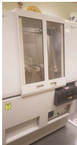
PANalytical X'Pert PRO CuK \alpha 1 – temperature programmed high resolution diffractometer (2008; D09/D10)
