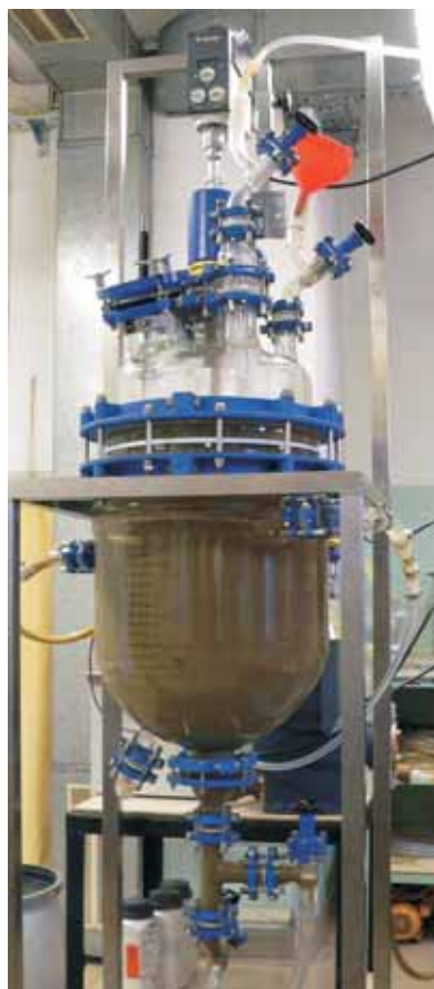
FIGURE 2: Anaerobic reactor for sludge treatment
