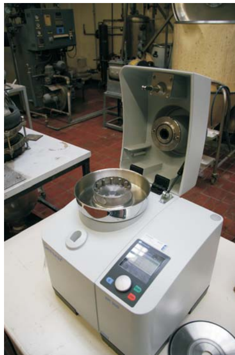
FIGURE 2: Combination of mills for disintegration of laboratory samples of biomass and mixed waste.
